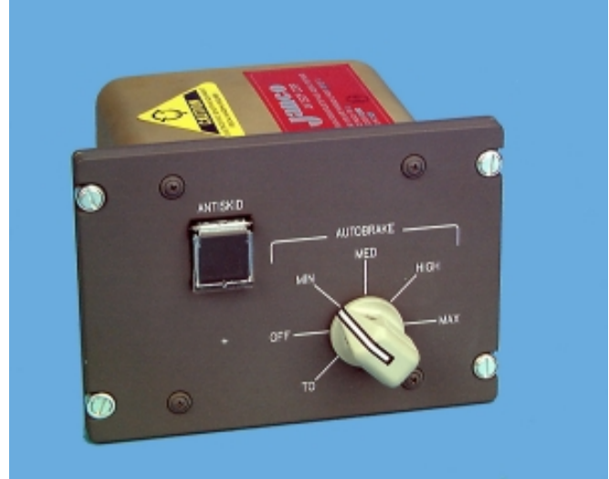
Figure 1, A Typical Autobrake Selector Panel (717)
