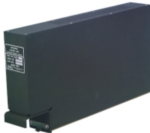
Figure 2, A Typical Autobrake Control Unit
